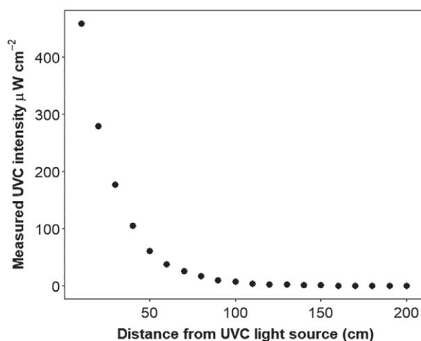
**Figure 2.** The maximum UVC irradiance (254 nm, 10 nm bandwidth) through seawater (salinity 34‰) at increasing distances, from three 11 W low pressure mercury lamps.
